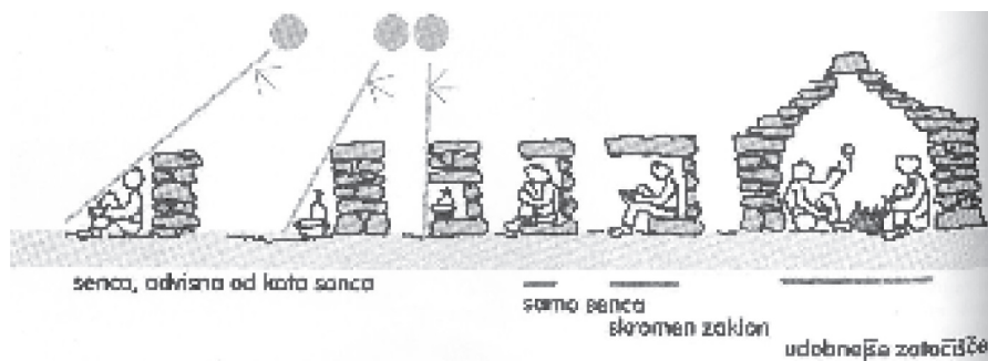
Fig. 2: Evolution from simple drystone wall to drystone cabin [2].
