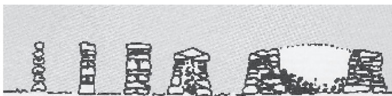
Fig. 1: Cross sections of different types of drywalls [2].
