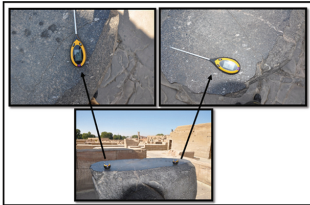
Pic. (2) Recording the temperatures of the outer surface of the granite rock in Kom Ombo Temple 2020.
