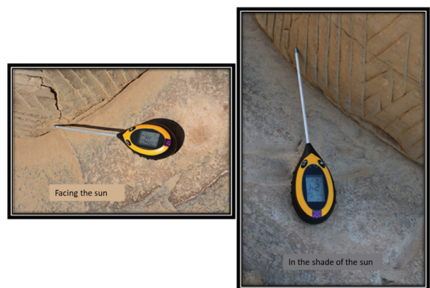
Pic. (1) The 4 in 1 Soil Survey instrument used to measure the surface temperature of the rocks in the temples of Kom Ombo and Philae2020.
