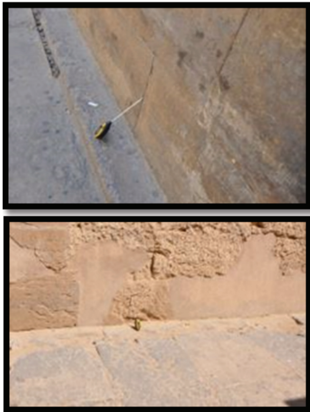
Pic. (4) Recording the temperatures of the outer surface of the rock in one of the walls of Kom Ombo Temple, site (3) 2020.
