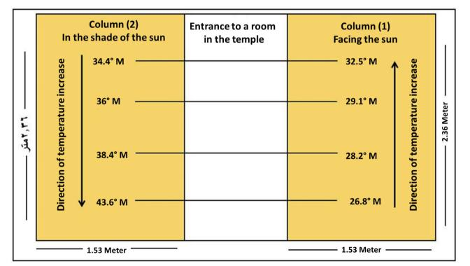
Source: The drawing was made based on a field study conducted by the student for the temple on 2/3/2020 Fig. (9) Illustration of a wall in Kom Ombo Temple showing the temperatures measured in the sector.
