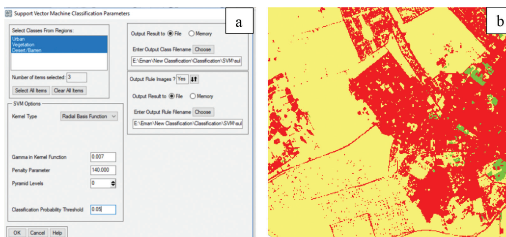
Figure 3 (a) An example of the parameters used in the process of SVM (error and trial phase), and (b) is the outcome, the colours represent: red is for urban areas, green is for the agricultural area, yellow is for the barren area,
